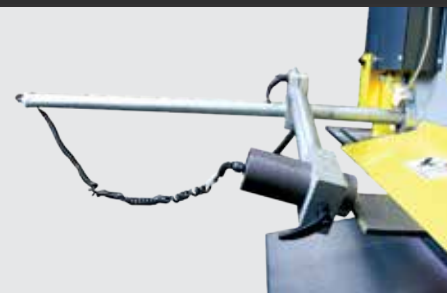
ELECTRIC BACK GAUGE
